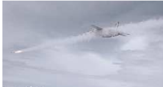
An F-14 Tomcat launches an AIM-9 sidewinder missile, a heat-seeking missile.
